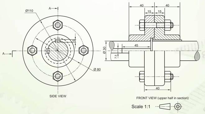
ASSEMBLED VIEWS OF AN UNPROTECTED FLANGE COUPLING
