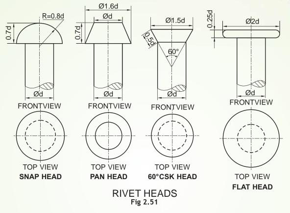
Example 23: Sketch freehand the Front view and Top view of a snap head rivet of diameter 20mm, keeping its axis vertical. Give standard dimensions.
