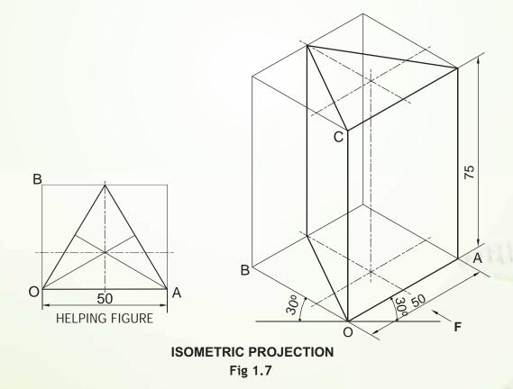
**Example 6:** An equilateral triangular prism of 50 mm base side and 70 mm long resting on one of its face on H.P. with axis of it perpendicular to V.P. Draw its isometric projection.
