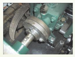
THE UNPROTECTED FLANGE COUPLING CONNECTS THE SHAFTS FROM A PUMP TO THAT OF A ENGINE Fig 6.3
