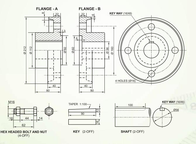
DETAILS OF A PROTECTED FLANGE COUPLING Fig 6.16
