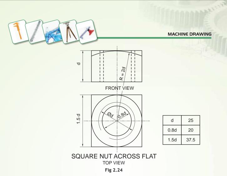
**Example 12:** Draw to scale full size the Front View and Top View of a square nut of diameter 25mm, keeping its axis vertical with the diagonal on the square face parallel to V.P.
