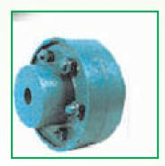
(a) Unprotected (b) Protected DIFFERENT TYPES OF FLANGE COUPLINGS Fig 6.2
