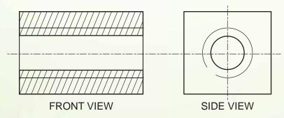
CONVENTIONAL REPRESENTATION OF INTERNAL V-THREADS Fig 2.38 ARRENTING &
