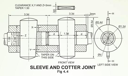
Question: Figure given below (fig: 4.5) shows the parts of a Sleeve and Cotter Joint. Assemble the parts correctly and then draw the following views to a scale 1: 1
