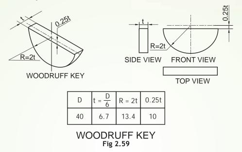
**Example 27:** Sketch freehand a woodruff-key in position, on a shaft of diameter 60mm, keeping the axis of the shaft parallel to V.P and H.P. Give standard dimensions.
