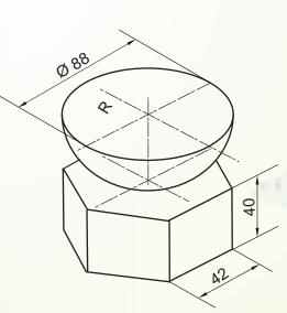
0. BELOW: HEXAGONAL SLAB. ABOVE: HEMISPHERE COMMON AXIS : VERTICAL
