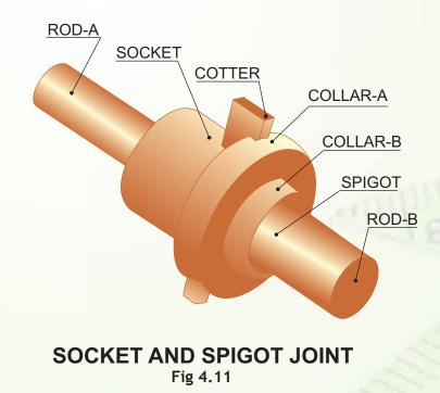
construction socket can be considered as a hollow pipe having one side solid and the other hollow, while the spigot is a solid rod, the solid spigot is nearly of the size of the internal radii of the socket, where it can fit. Once they are fit, consider that a rectangular cavity of tapering construction through both the parts, i.e., spigot and socket. This cavity or slot is kept slightly out
