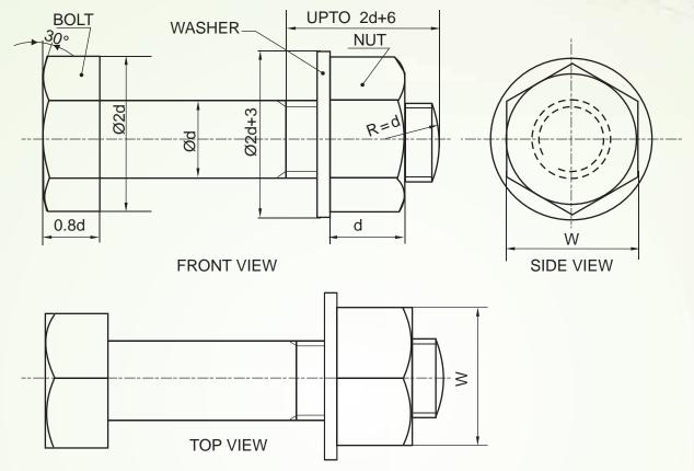
COMBINATION OF HEXAGONAL HEADED BOLT WITH HEXAGONAL NUT & WASHER Fig 2.29
