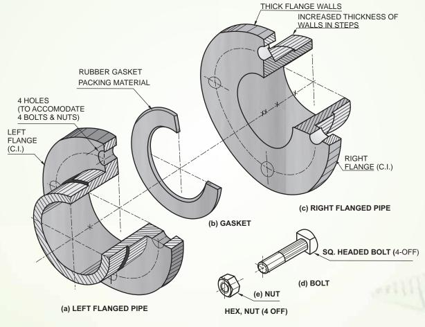
DETAILS OF A FLANGE PIPE JOINT (HALF SECTIONAL PICTORIAL VIEW) Fig. 5.13
