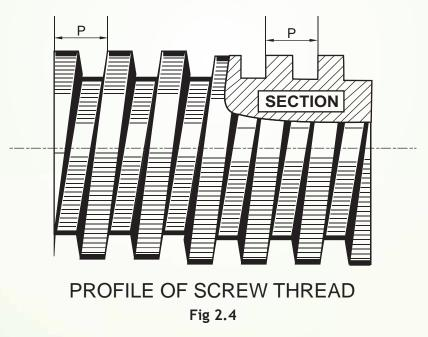
The section of a thread cut by a plane containing the axis is known as the form of the screw thread. It is also called the profile of the thread. Refer FIG 2.4
