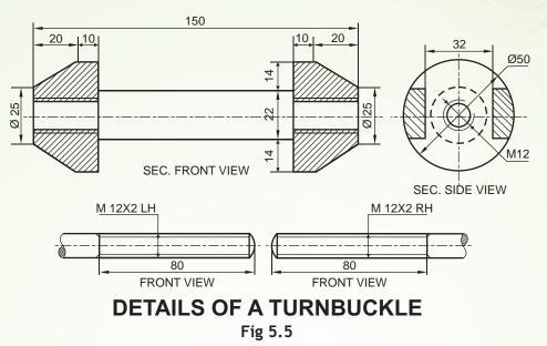
**Solutions:** The above fig 5.5 shows orthographic views of different parts of a `Turnbuckle". Let us assemble them correctly to obtain/ draw the required views.
