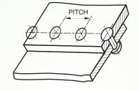
SINGLE RIVETED LAP JOINT. Fig, 2.33
