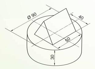
5. BELOW: CIRCULAR SLAB 6. ABOVE: EQUILATERAL TRIANGULAR PRISM AXIS: VERTICAL AND HORIZONTAL
